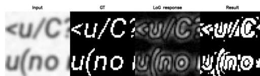
Fig. 31. Example of the best Laplacian of Gaussian result on the test subset using Gaussian kernel size = 7, sigma = 1.5, and LoG threshold = 40
