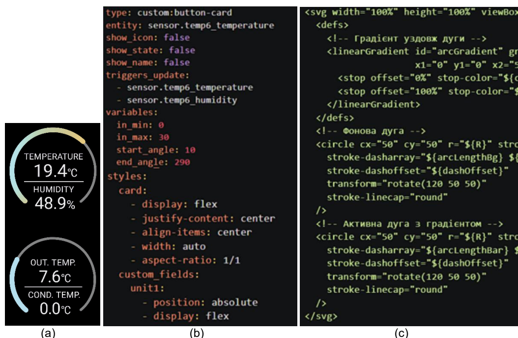
Fig. 4. Implementation of data visualization using Custom Button Card (a), YAML configuration (b), and SVG graphics (c).
