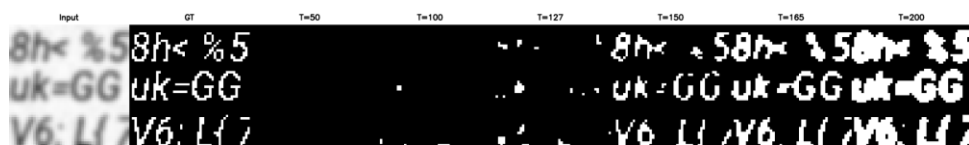
Fig. 4. Visual comparison of simple thresholding results with different threshold values on a test image
