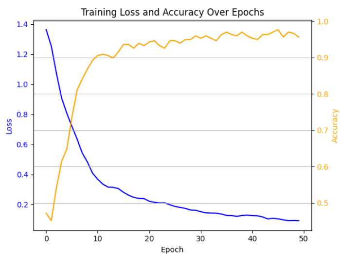
Fig. 4. Loss and accuracy over epochs for KAN (3, 64, 64, 4).
