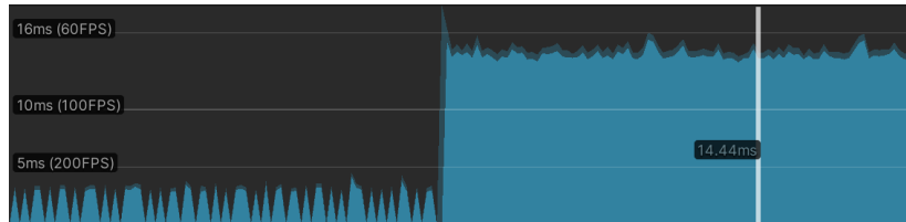
Fig. 5. Increasing rays count to 100 per frame with 8 bounces still took less than 16 ms of computational time
