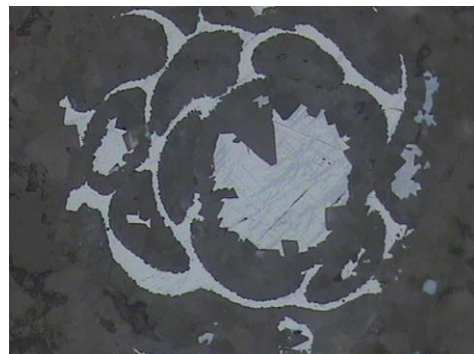
Fig. 9. Low temperature intergrowth of sphalerite (grey) with galena (white) and chalcopyrite in dolomite sparite, Rudna Mine.
