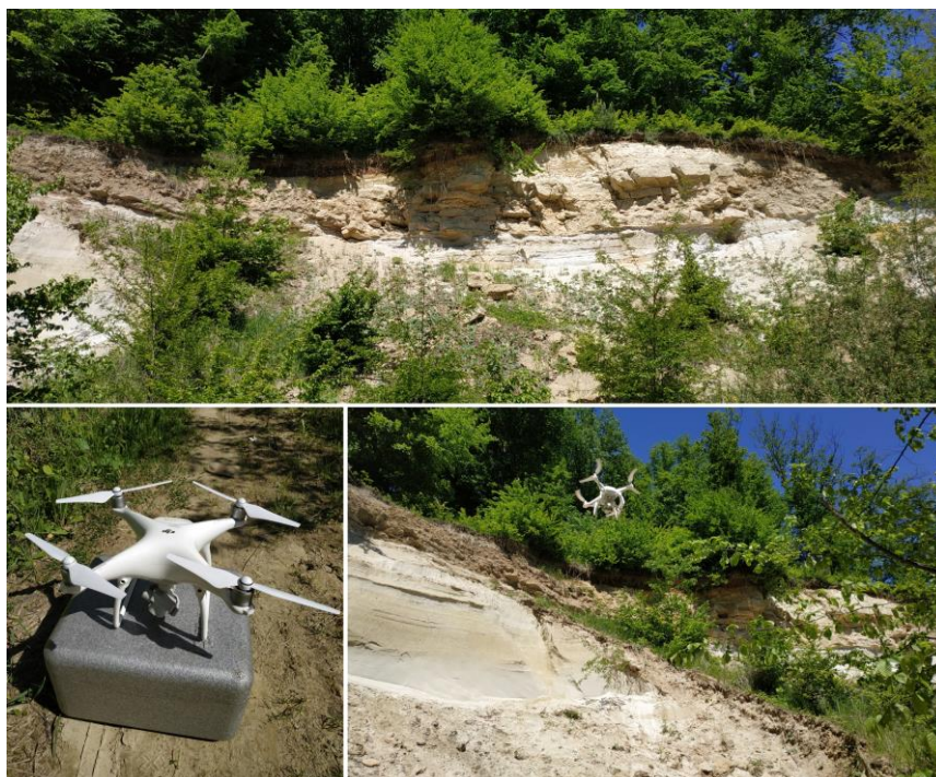
Fig. 5. Geological survey of Miocene rocks by drone Phantom 4
