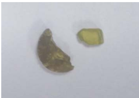
Fig. 1. Appearance of \text{Tl}_4\text{CdI}_6 single crystal grown with a Bridgman–Stockburger technique.
