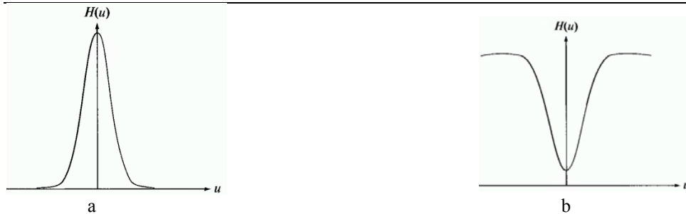
Fig. 1. (a)-Gaussian frequency domain Lowpass filter and (b) - Gaussian frequency domain Highpass filter.
