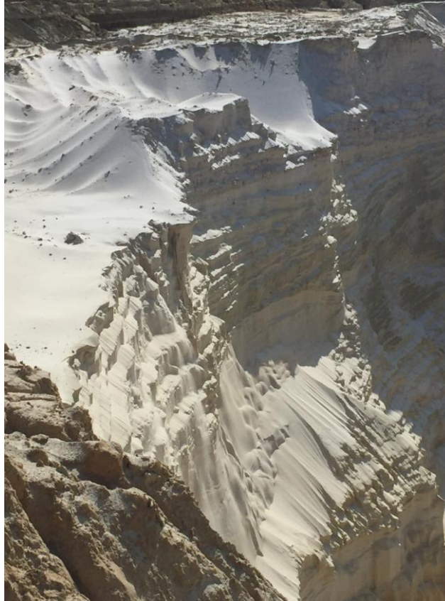
Fig. 8. The combination of scree formation and aeolian processes (the Davydivskiy Quarry № 1)
