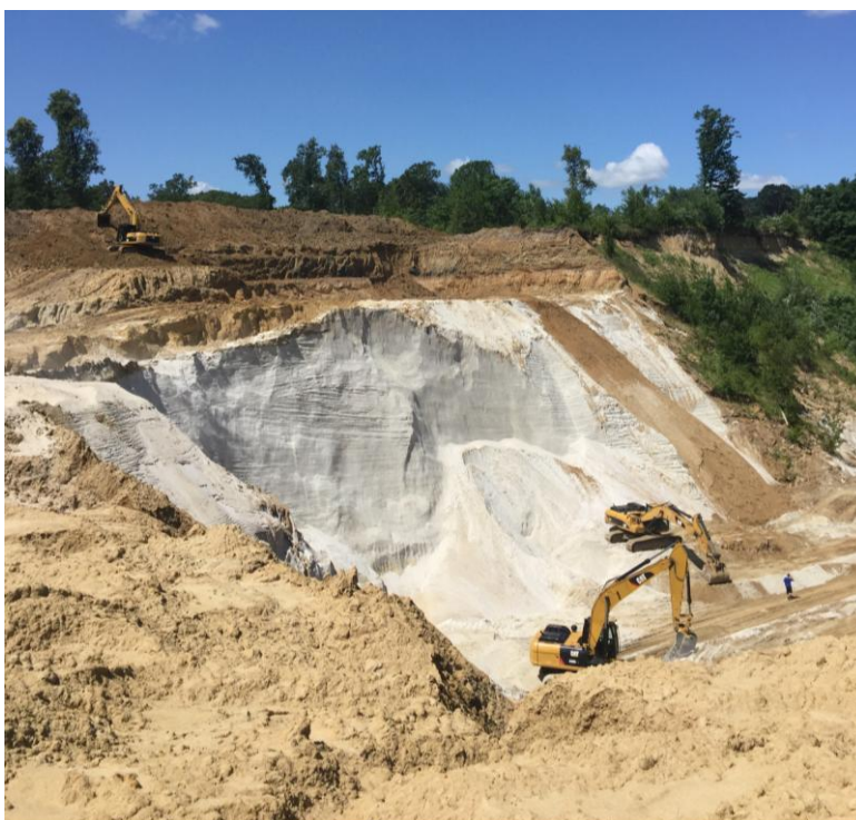
Fig. 7. Scree formation and water-erosion processes in the Davydivskyi Quarry № 1
