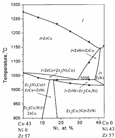
**Fig. 4** The Zr<sub>57</sub>Co<sub>43</sub>–Zr<sub>57</sub>Ni<sub>43</sub> section.
