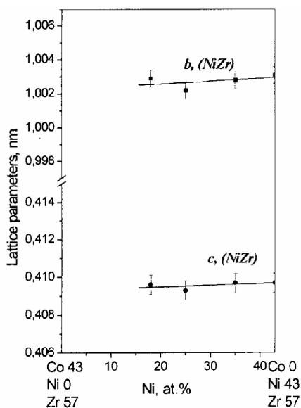
Fig. 3 Composition dependence of the lattice parameters in  $Zr_{57}Co_{43}$ – $Zr_{57}Ni_{43}$  alloys.
