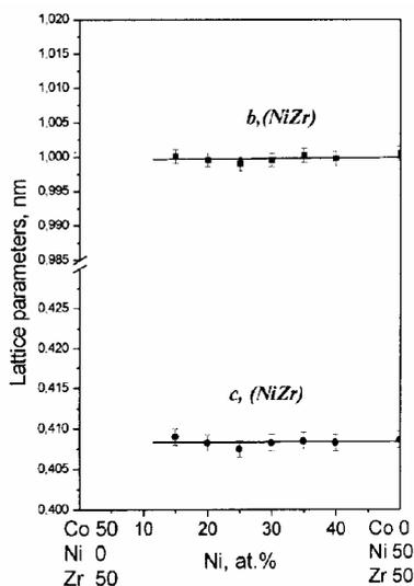
Fig. 1 Composition dependence of the lattice parameters in ZrCo–ZrNi alloys.
