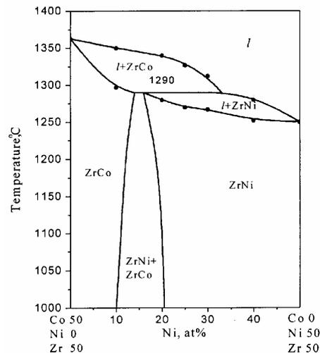
Fig. 2 The ZrCo–ZrNi section.
