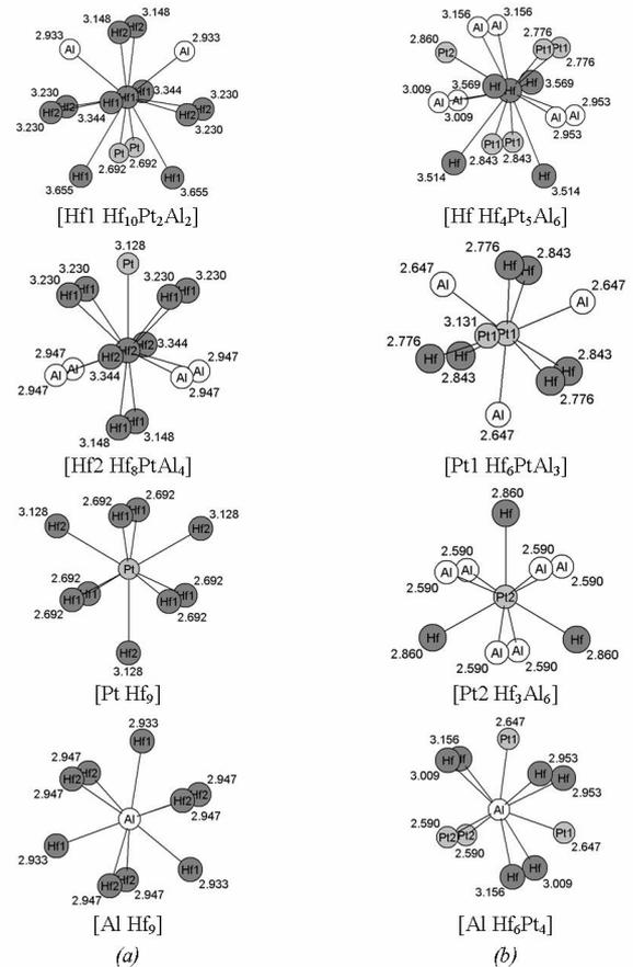
**Fig. 3** Nearest-neighbor environments in the structures of Hf<sub>6</sub>PtAl<sub>2</sub> (a) and HfPtAl (b). Coordination polyhedra of the central atoms are indicated. Interatomic distances are shown in Å.
