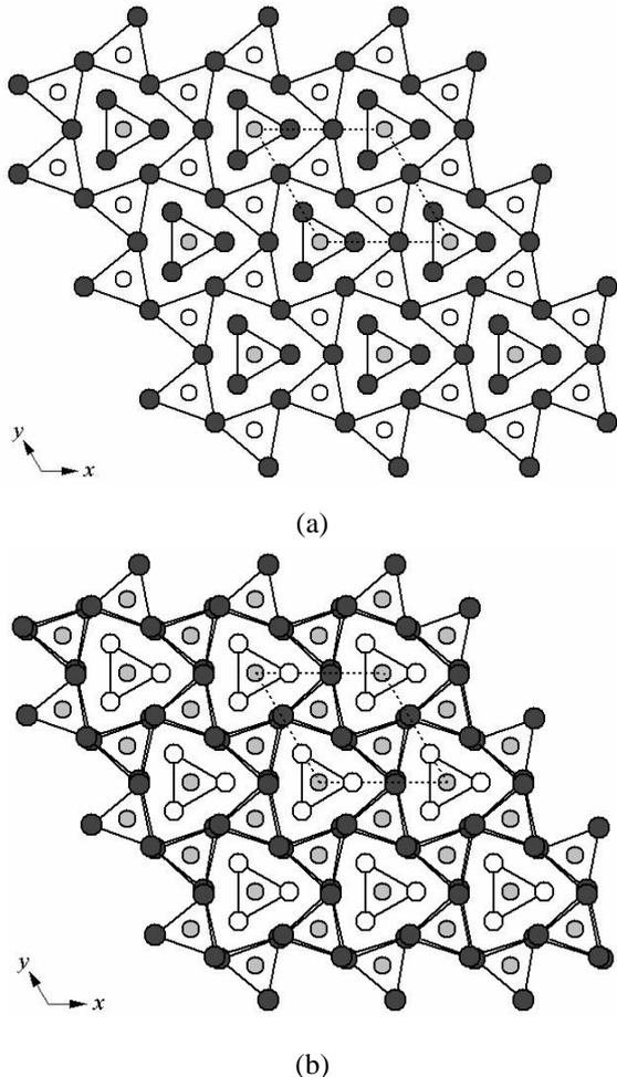
**Fig. 2** Projections of the structures of Hf<sub>6</sub>PtAl<sub>2</sub> (a) and HfPtAl (b) on the *xy* plane. Black circles indicate Hf atoms, grey filled circles are Pt atoms, and Al atoms are represented by white circles. The unit cells are shown using dotted lines.
