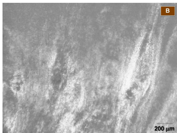
Fig. 1 Textures observed with the aid of a polarizing microscope for pure \text{Cd}(\text{C}_7\text{H}_{15}\text{COO})_2 mesophase (a) and a mixture with copper nanoparticles (b) at 150°C.
