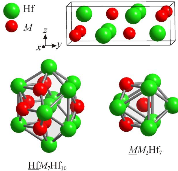
**Fig. 2** Unit cell and coordination polyhedra of the atoms in the structure of  $\text{HfGa}_{0.33}\text{Si}_{0.67}$ .
