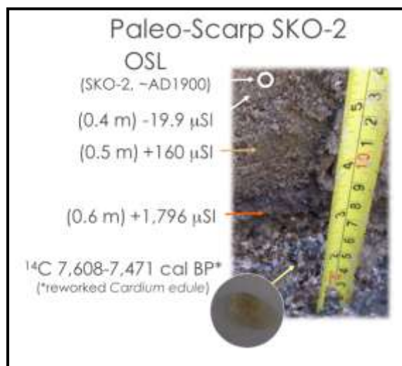
Fig. 4. Trench through paleo-scarp SKO-2 (right side of profile in Fig. 3) shows an extreme concentration of heavy minerals with MS values nearly 20x higher than that of the recent beach (see Fig. 2). Such anomalies not only serve as prominent reflections in GPR images (Fig. 3), helping locate, map, and characterize HMCs geometry, but can provide quantitative information about near-surface shear stress of the flow responsible for their formation. Note the early Holocene age of the reworked mollusk, which provides information on the nearshore sediment source, but not the erosional event. The optical age of ~100 years likely post-dates the scarp, but is much closer to the age of the storm event.
